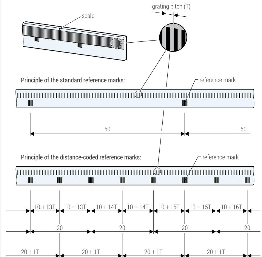
These incremental linear encoders work according to an imaging photoelectric measuring principle with a transmissive **singlefield scanning**.
