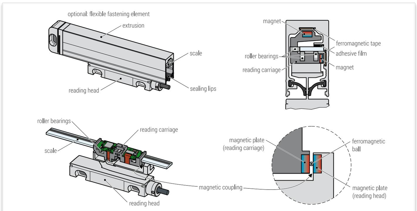
A high accuracy grating is deployed as scale graduation. Depending on the model, glass ( $\alpha \approx 8,5 \times 10^{-6}/K$ ) or glass ceramics ( $\alpha \approx 0 \times 10^{-6}/K$ ) is employed as base.
