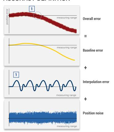
The accuracy of a linear encoder is mainly determined by the baseline error of the scale unit, the interpolation error of the optoelectronic scanning and the position noise.
