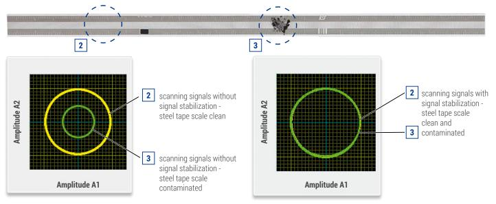
Effect of contamination on the intepolation error Steel tape scale contaminated by fluids, dust, particles, fingerprints etc.
