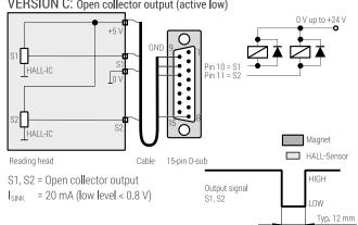
According to factory default setting the actuator magnets are placed at the beginning (S1) and at the end (S2) of measuring length and can be moved by the customer.
